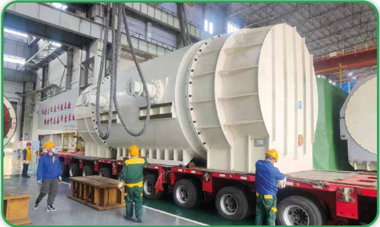
Generator - Loading at China Factory
